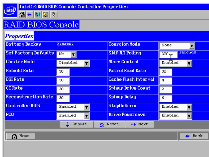
**Figure 62. Additional Controller Properties**
