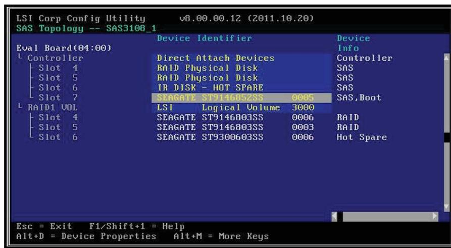
**Figure 14. Boot Device on SAS Topology Window**
